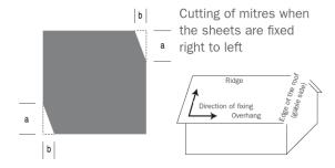
A = according to sheet over lap + 5 mm B = 50 mm
