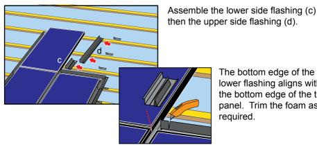
The bottom edge of the lower flashing aligns with the bottom edge of the top panel. Trim the foam as required.
