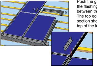
Push the gutter extension (a) into the flashing gasket across the join between the two left hand panels. The top edge of the full gutter section should be aligned with the top of the lower panels.
