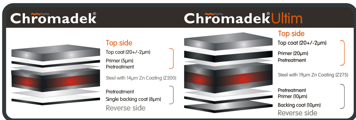
Figure 1: Coating configuration of Chromadek® Standard and Chromadek ULTIM®.
